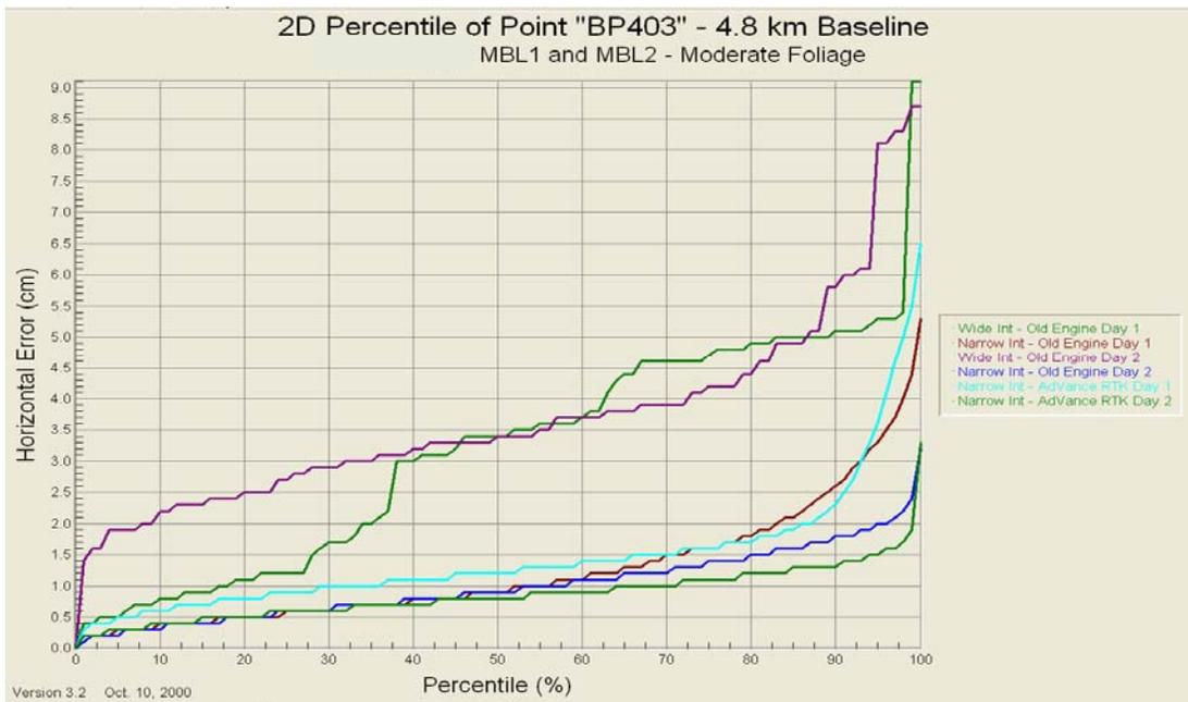
**Figure 11: Both Engine's Position Error at 4.8 km Baseline**
