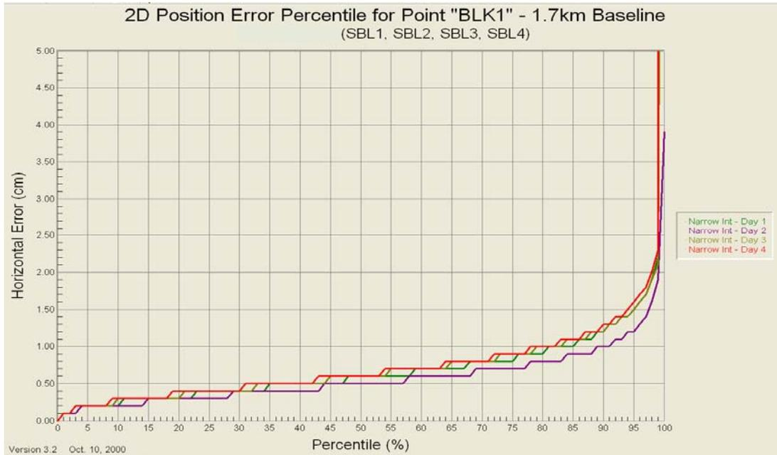
**Figure 10: AdVance RTK Position Error at 1.7 km**
