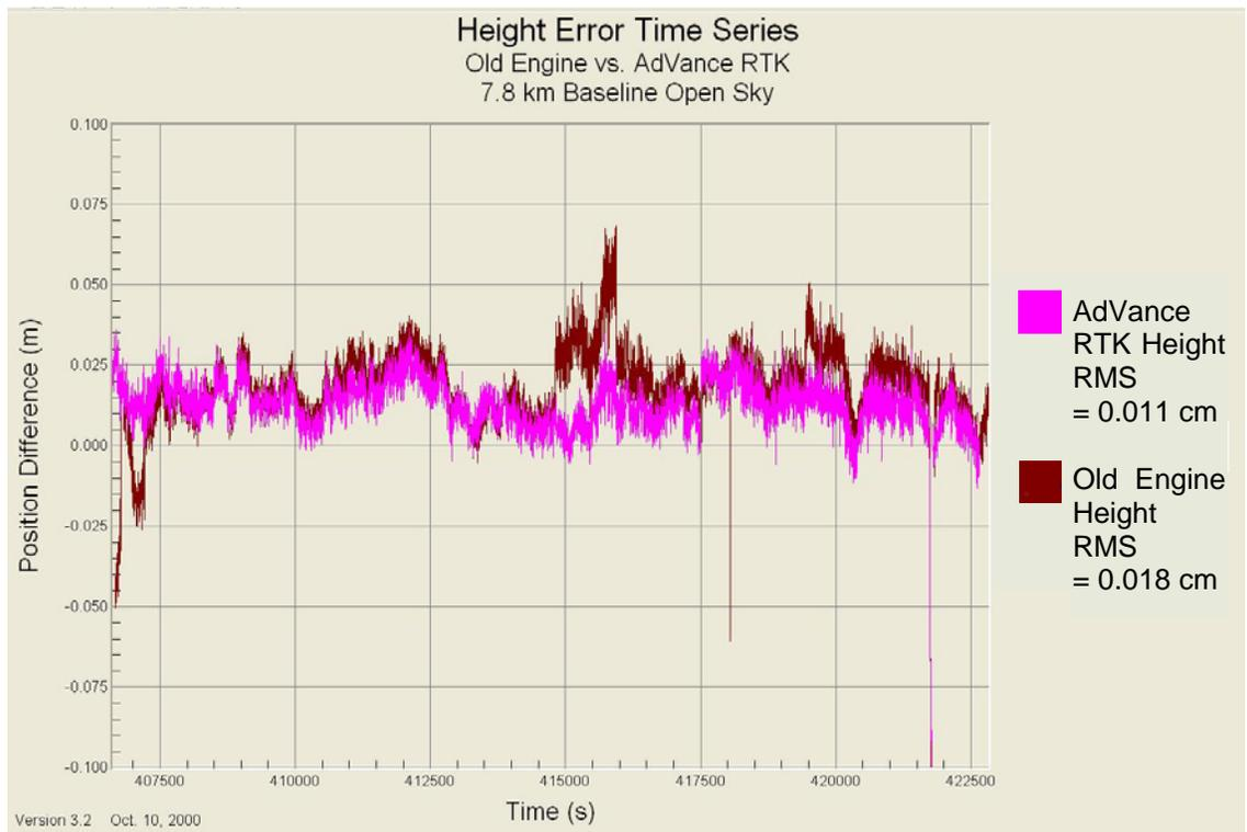
**Figure 7: Old Engine vs AdVance RTK Height Error**
