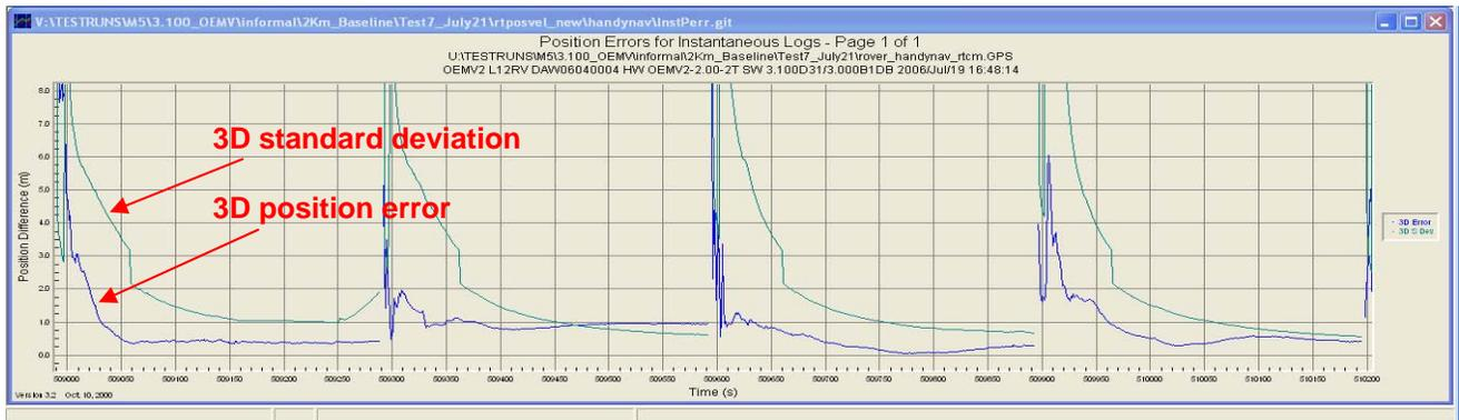
Figure 13: AdVance RTK Engine's Position Difference in Foliage
