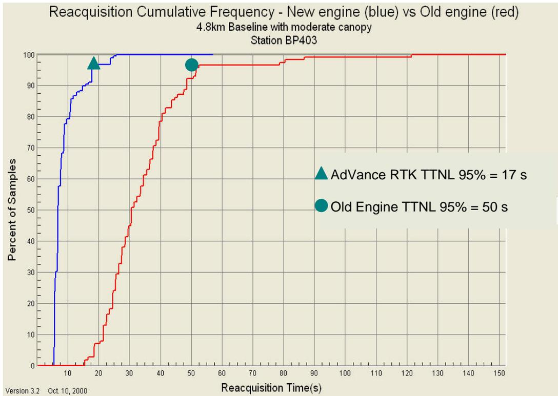
**Figure 5: Reacquisition Time Under Moderate Canopy**
