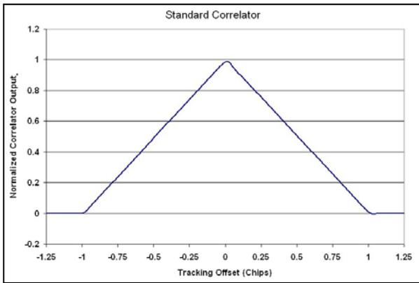
**Figure 1 Standard correlation output of GPS Prn1**
