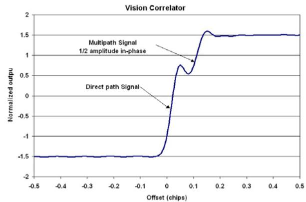
Figure 7 Vision Correlator with 1/2 amplitude MP at 0.1 chip delay, in-phase
