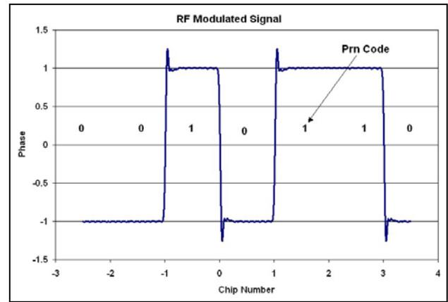
**Figure 2 Time domain simulation of the In-phase channel of a GPS receiver**
