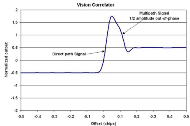
Figure 8 Vision Correlator with 1/2 amplitude MP at 0.1 chip delay, out-of-phase
