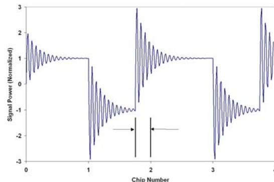
**Figure 19 Threat Model C Unbalanced Duty cycle and RF Ringing**
