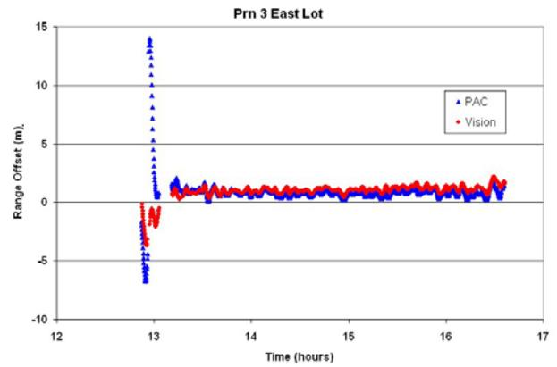
**Figure 13 Typical satellite pass (Prn 3 East parking lot)**
