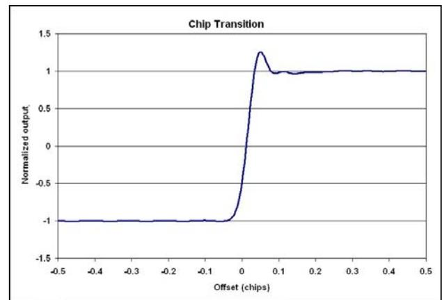
**Figure 3 Average chip transition of GPS PRN 1 as measured using NovAtel ME3 GNSS receiver**
