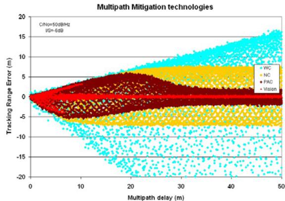
**Figure 10 Comparison of multipath processing techniques**
