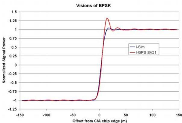
**Figure 9 Reference function from GPS PRN 21 and STR4760**
