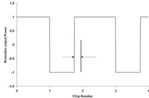
**Figure 17 Threat Model A Unbalanced Duty cycle**
