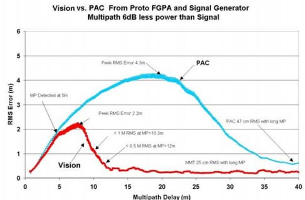
**Figure 11 RMS errors of Vision and PAC multipath performance**
