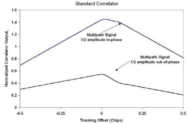
Figure 6 Standard Correlator with 1/2 amplitude MP at 0.1 chip delay, in-phase and out-of-phase
